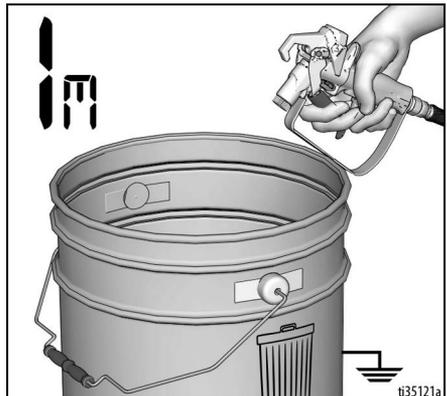
8. Move gun to paint pail and trigger for 20 seconds. Release trigger and allow sprayer to build pressure. Engage trigger lock.
