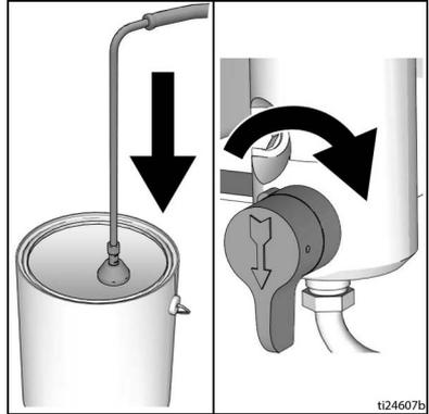
5. Hold a metal part of the spray gun firmly to a grounded metal pail. Point spray gun into pail. Disengage the trigger lock and trigger the spray gun to relieve pressure.
