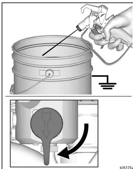
6. Turn pressure control to Fast Flush operate until the pump runs steady and flushing fluid appears in the waste pail.
