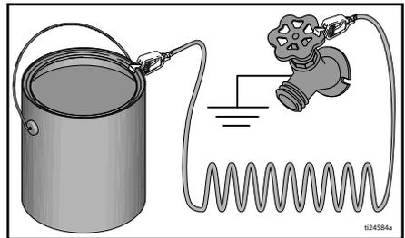
**To maintain ground continuity when sprayer is flushed or pressure is relieved:** hold metal part of spray gun firmly to the side of a grounded metal pail then trigger the gun.
