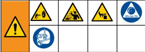
This equipment stays pressurized until pressure is manually relieved. To help prevent serious injury from pressurized fluid, such as skin injection, splashed fluid and moving parts, follow the Pressure Relief Procedure whenever sprayer is stopped and before sprayer is cleaned or checked, and before equipment is serviced.
