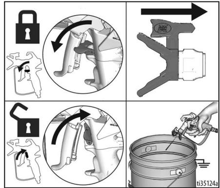
2. Engage trigger lock. Return Spray Tip to original position. Disengage trigger lock and continue spraying.
