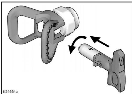
4. Screw assembly onto gun. Tighten.
