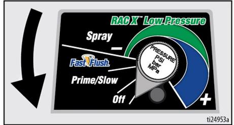
4. Put drain tube in a pail and turn prime valve down to relieve pressure. Leave prime valve in the down (drain) position until you are ready to spray again.
